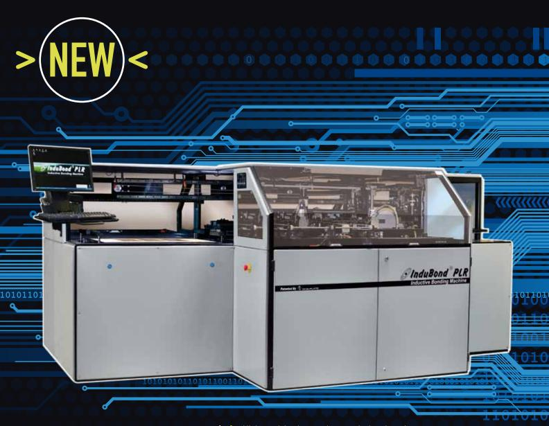
InduBond®, High Accuracy Optical Registration System for Pin Less Lamination
